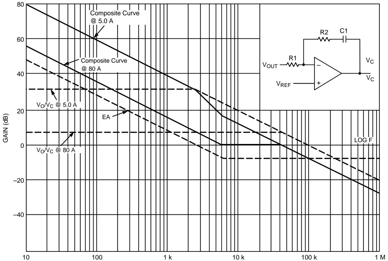
Figure 9. Frequency Response Diagram for Power Supply. Inset E/A Configuration
