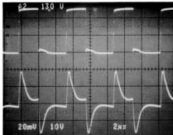
Figure 12.  $V_{DS}(\text{Top})$ ,  $I_D(\text{Bot.})$  (2.0 A/div) High Load
