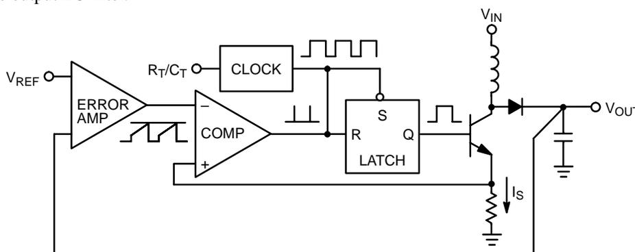
Figure 1. Basic Circuit Using Current-Mode Control
