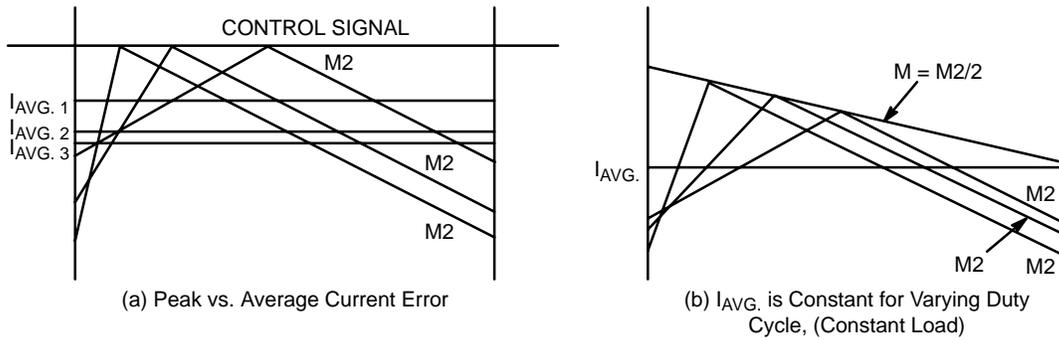
**Figure 2. Peak Current Detection is Used to Keep  $I_{AVG}$  Constant for Varying Duty Cycles**
