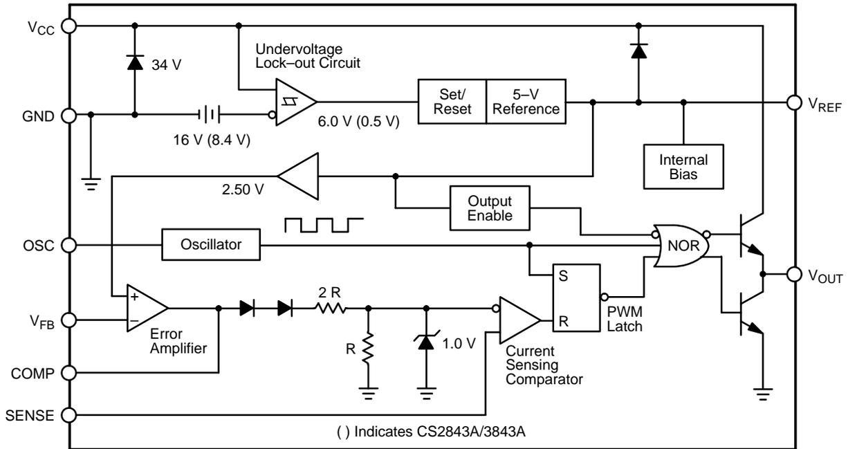
**Figure 3. CS3842A/3843A Block Diagram**
