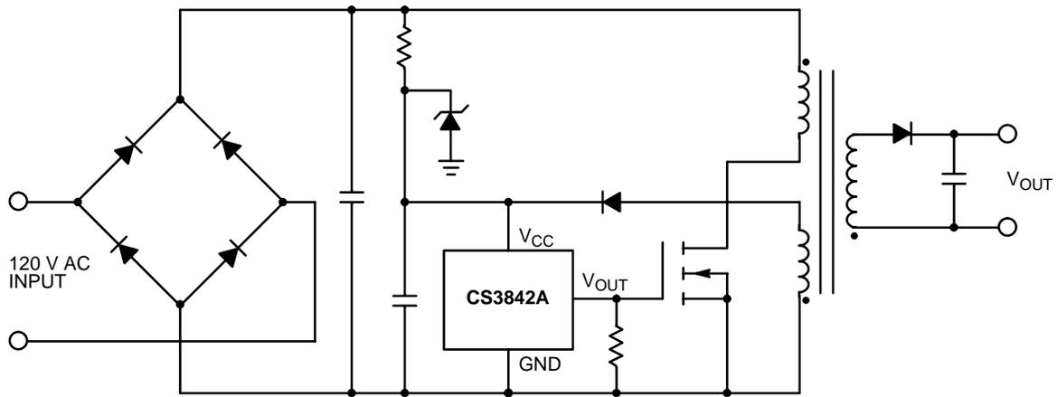
Figure 4. Common Off-Line Operation of CS3842A
