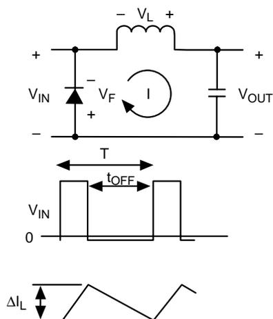
Figure 8. The Output Filter Circuit
