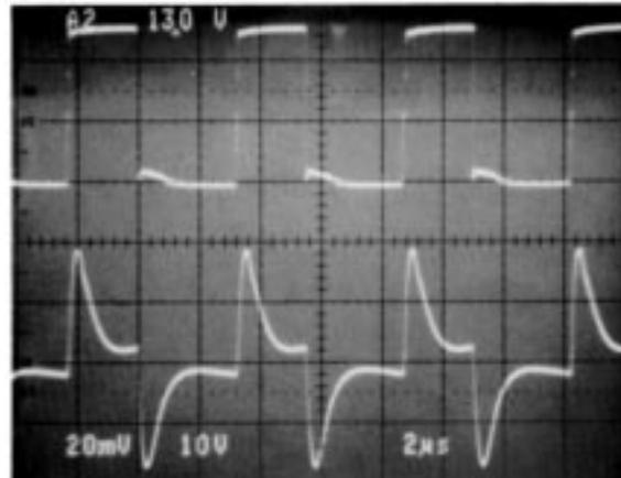
Figure 11.  $V_{DS}(\text{Top})$ ,  $I_D(\text{Bot.})$  (0.5 A/div) Low Load
