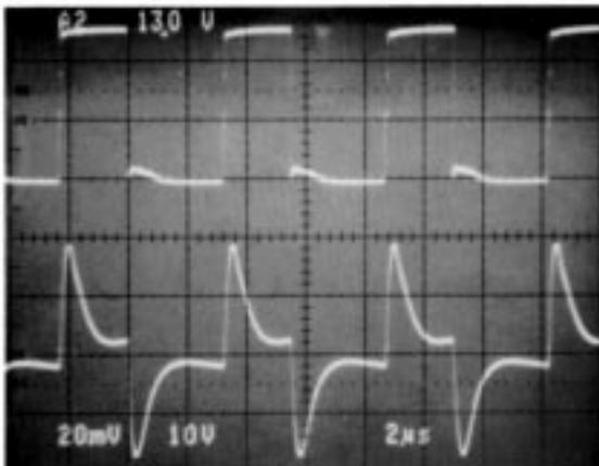
Figure 10. CS3842A Output Voltage and Current (200 mA/div)
