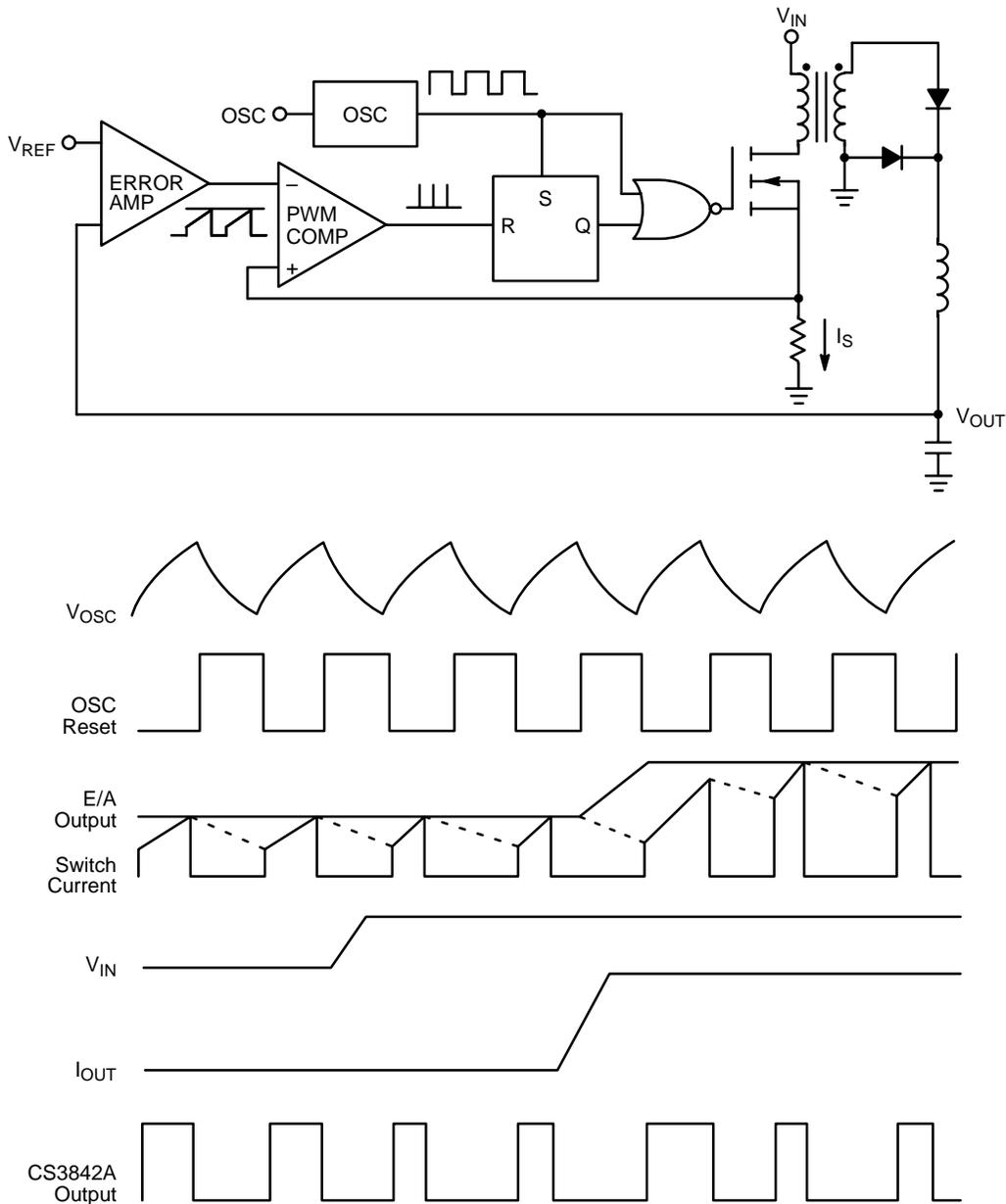
Figure 6. CS3842A Typical Waveforms
